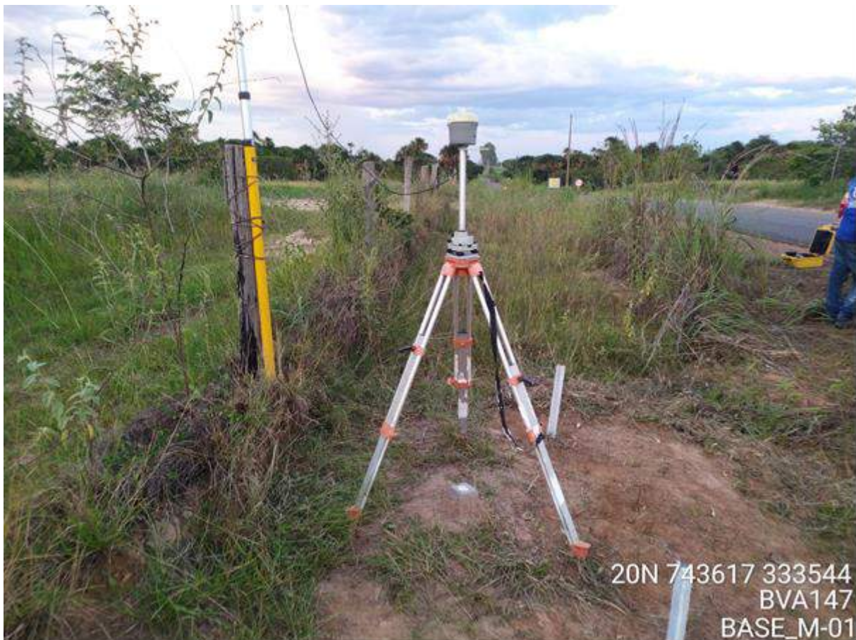
Receptor GNSS CHC i80, base, marco M-01 na BVA147.
